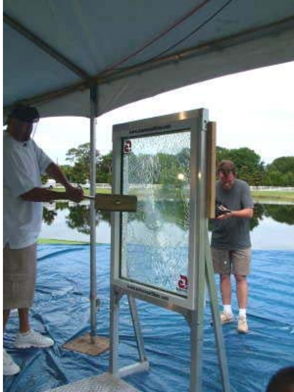
That is Matt Geiger, former NBA player, striking a window that has been protected with security window film. The photo was taken the instant just after the mallet bounced off the glass. The glass shattered, but did not fall to the ground. It was held in place by the durable and crystal-clear window film. PHOTO CREDIT: Tim Carter
