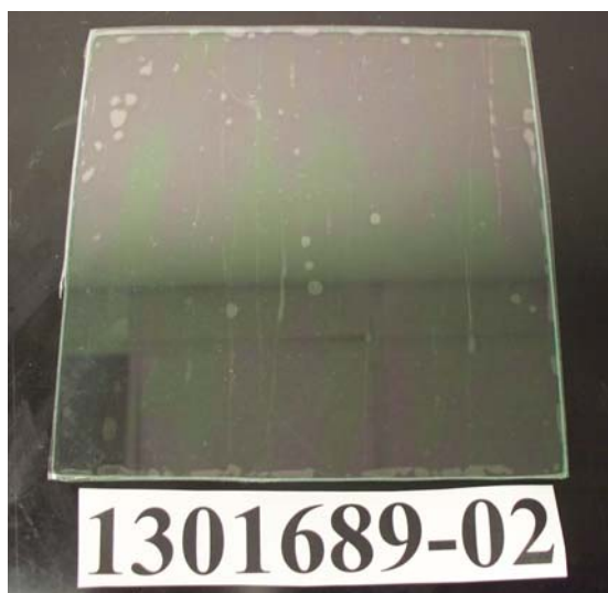
Solar Gard® Safety Window Film with Pressure Sensitive Adhesive as tested
