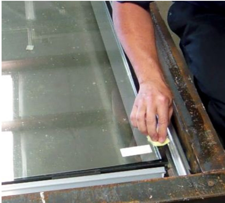
Photo#1 Specimen #1 Pentagon Flexible Membrane Specimen Perimeter of All Film Edges Treated with an Adhesion Promoter (3M 4298)
