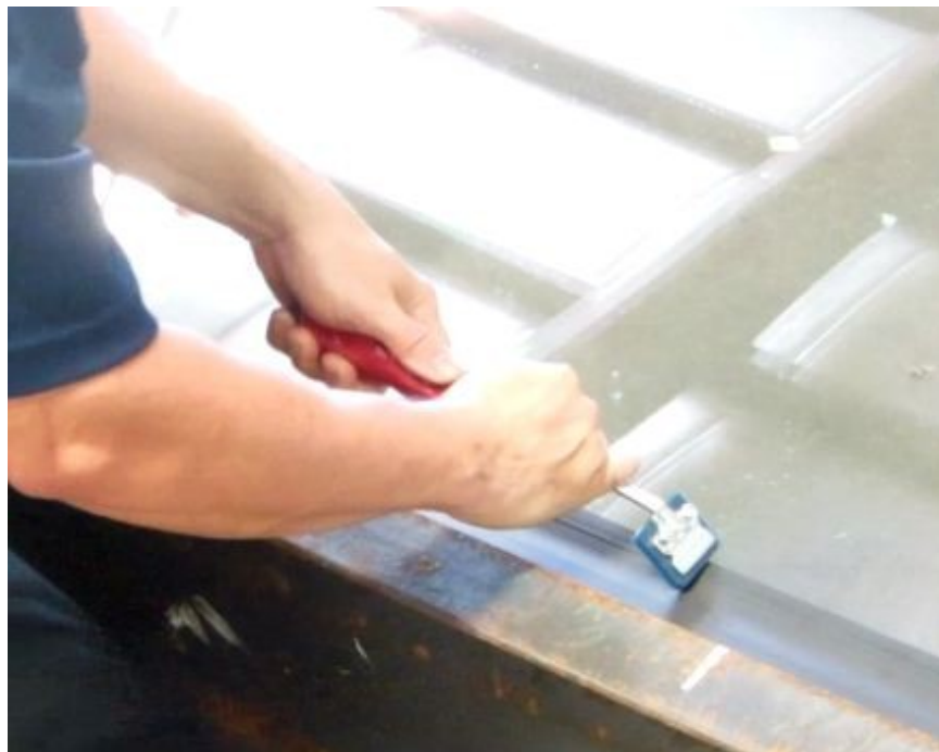
Photo#4 Specimen #1 Pentagon Flexible Membrane Specimen The Pentagon Flexible Membrane Secured in Place to the Film by Applied Pressure Using Application Tools. Application Tool #2
