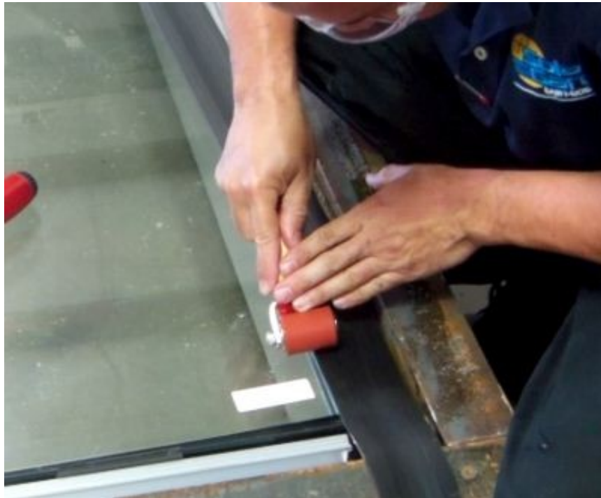
Photo#3 Specimen #1 Pentagon Flexible Membrane Specimen Pentagon Flexible Membrane Secured in Place to the Film, by Applied Pressure Using Application Tools. Application Tool #1
