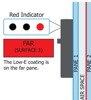
The RED light indicates that a LOW-E coating exists on a FAR surface of the window. The far surfaces of the window are surface #3 or #4 as you look at the window.
