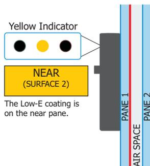
The YELLOW light indicates that a LOW-E coating exists on the NEAR surface of the window. The near surface of the window is surface #2 as you look at the window.
