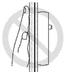
Placing your hand or an object on the opposite side of the window may cause improper results. Remove hand or object.
