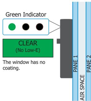
The GREEN light indicates that the window is CLEAR of any LOW-E COATING. NO LOW-E coating exists on any of the surfaces
