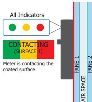
When the ETEKT+ is in direct contact with a LOW-E coating the GREEN, YELLOW and RED indicators will all be lighted.
