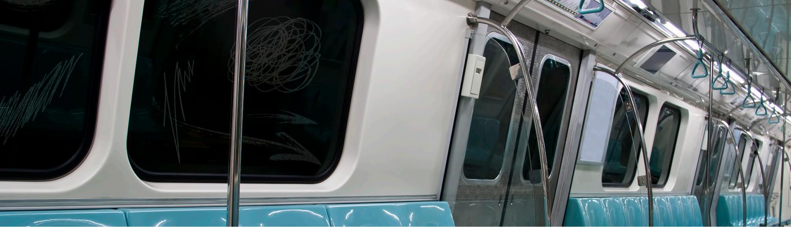
Glass surfaces are common targets for taggers using various tools to scratch or etch their 'art' leaving sometimes irreparable damage. Replacement or repair options can be time consuming and very costly.
