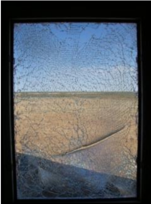
Figure C.13: Specimen 2 Internal Post-Blast Condition
