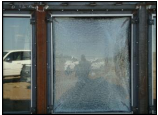
Figure C.22: Specimen 14 External Post-Blast Condition
