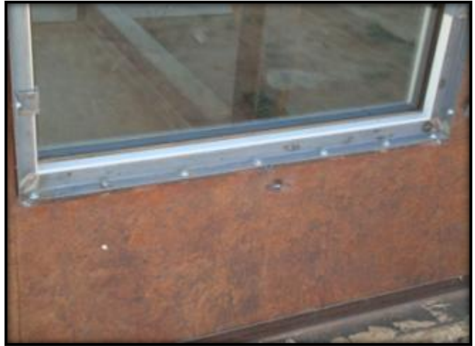
Figure C.2: L1 Bolt Connection Pre-Blast Condition
