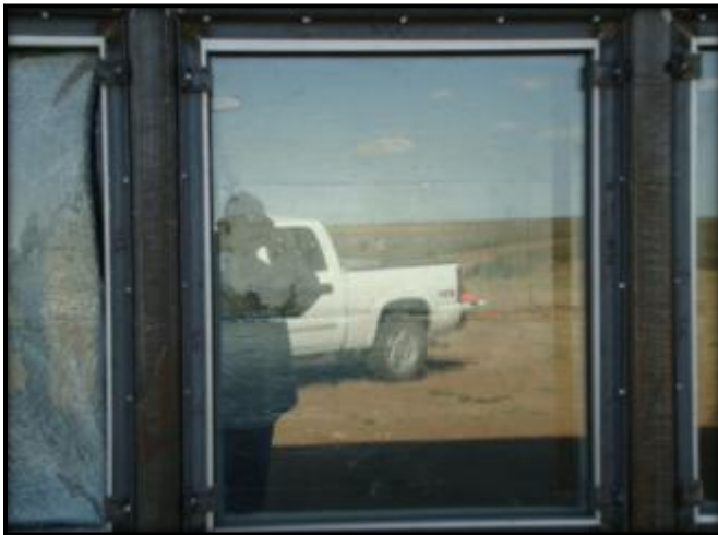
Figure C.23: Specimen 15 External Post-Blast Condition
