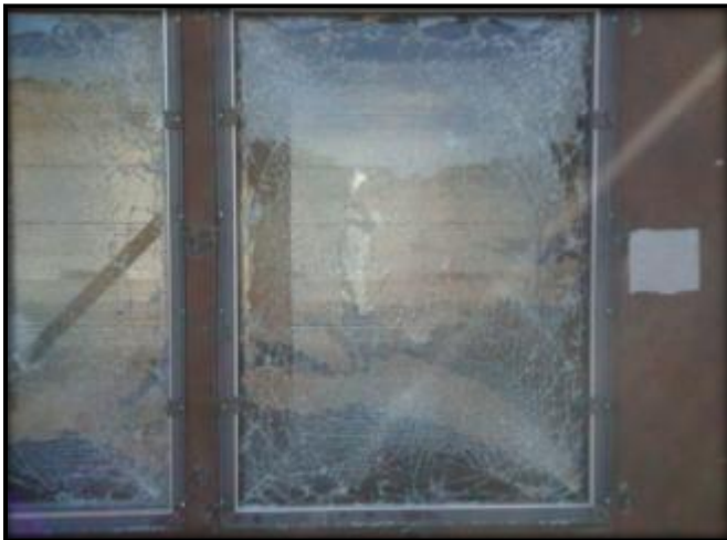
Figure C.11: Specimen 4 External Post-Blast Condition
