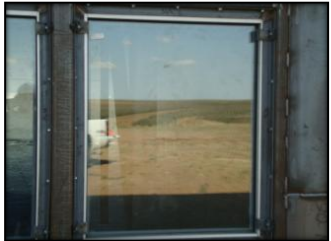
Figure C.24: Specimen 16 External Post-Blast Condition
