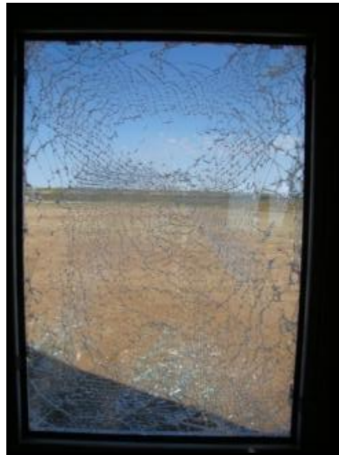
Figure C.12: Specimen 1 Internal Post-Blast Condition
