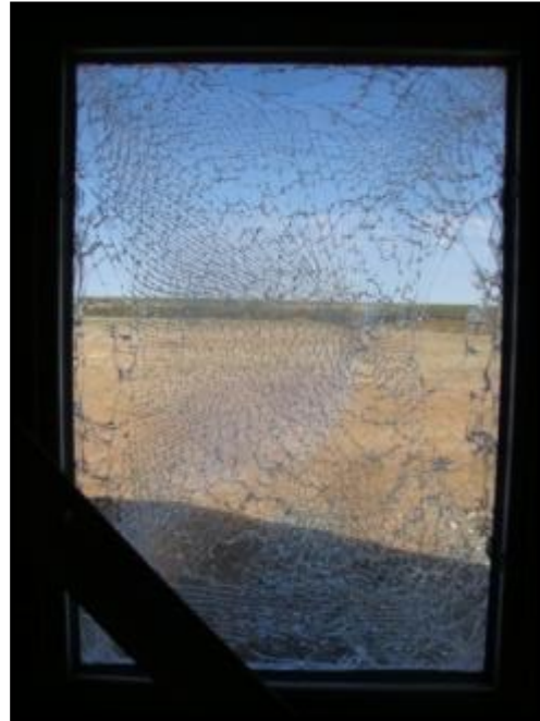
Figure C.14: Specimen 3 Internal Post-Blast Condition
