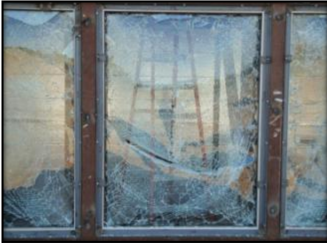
Figure C.9: Specimen 2 External Post-Blast Condition
