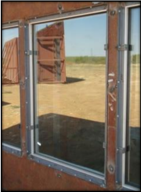
Figure C.5: Specimen 3 Pre-Blast Condition
