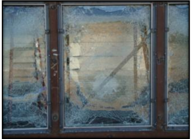
Figure C.10: Specimen 3 External Post-Blast Condition
