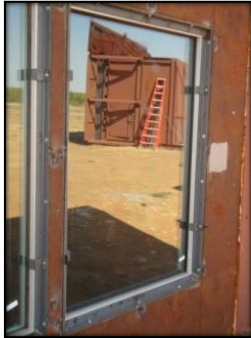
Figure C.6: Specimen 4 External Pre-Blast Condition
