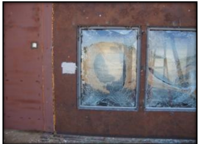
Figure C.8: Specimen 1 External Post-Blast Condition
