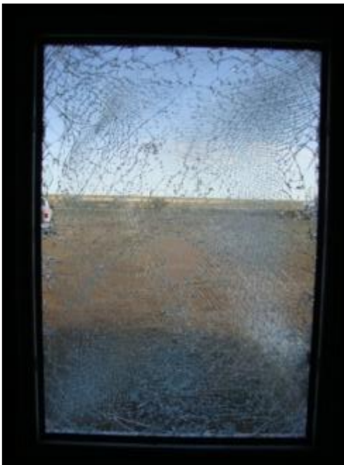
Figure C.15: Specimen 4 Internal Post-Blast Condition
