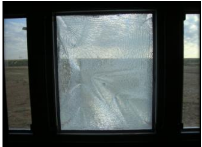
Figure C.28: Specimen 14 Internal Post-Blast Condition
