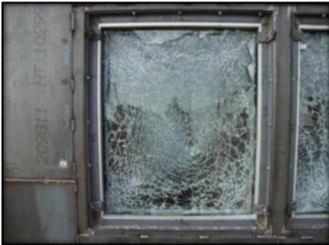
Figure C.11: Specimen 9 External Post-Blast Condition
