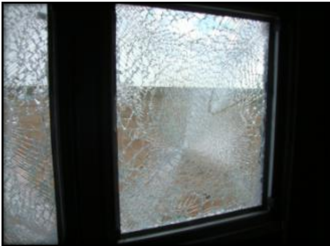
Figure C.15: Specimen 9 Internal Post-Blast Condition
