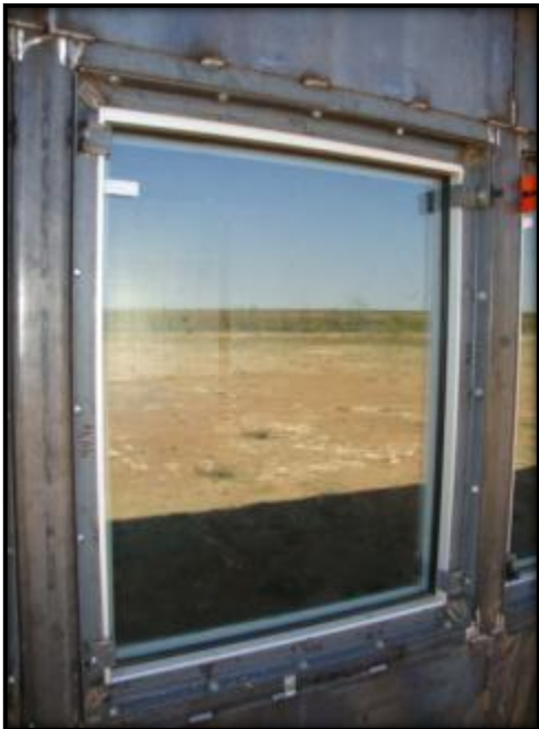
Figure C.3: Specimen 11 Pre-Blast Condition
