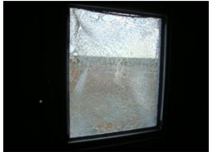
Figure C.18: Specimen 12 Internal Post-Blast Condition
