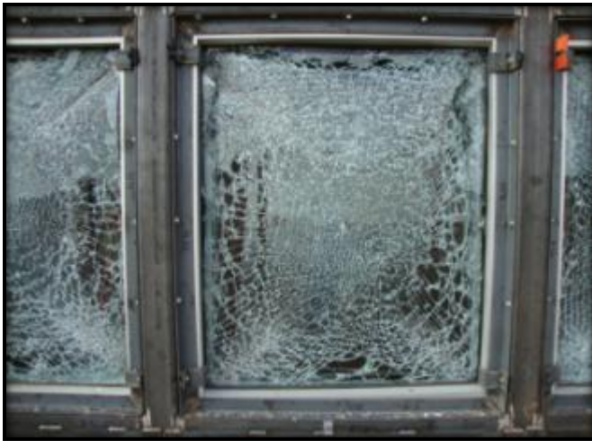
Figure C.13: Specimen 11 External Post-Blast Condition
