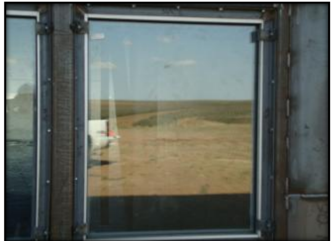
Figure C.26: Specimen 16 External Post-Blast Condition
