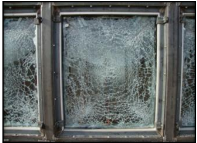
Figure C.12: Specimen 10 External Post-Blast Condition
