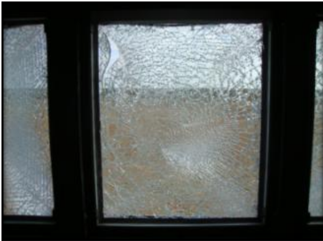
Figure C.17: Specimen 11 Internal Post-Blast Condition
