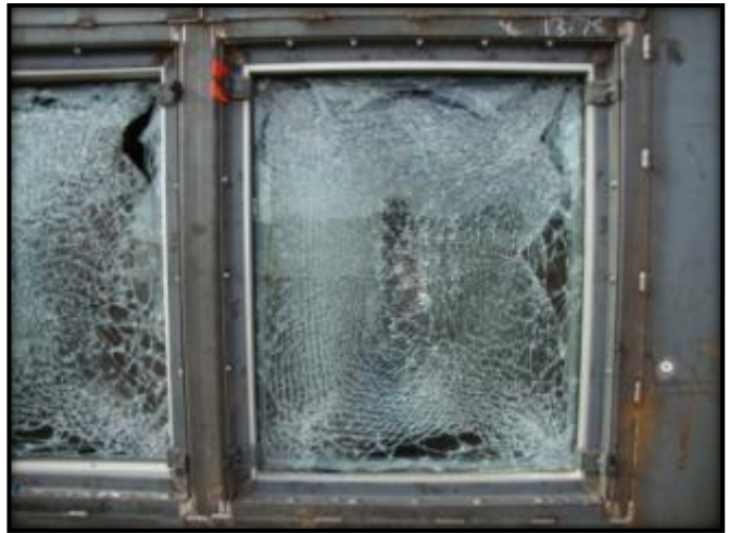
Figure C.14: Specimen 12 External Post-Blast Condition
