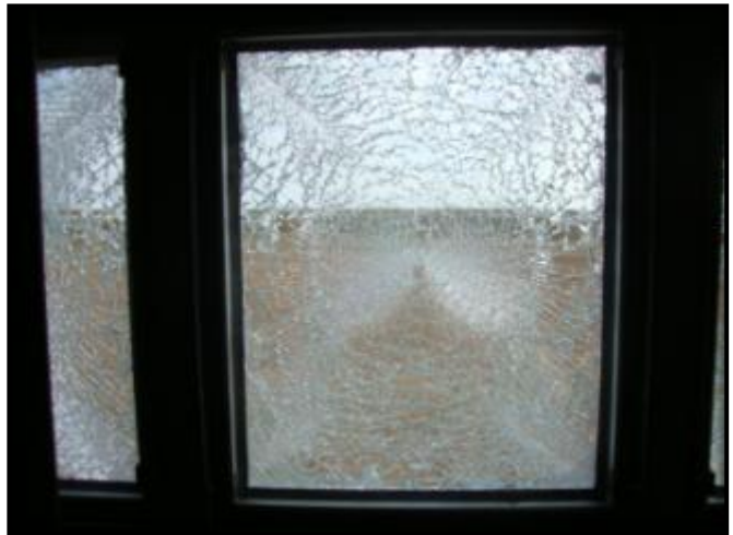
Figure C.16: Specimen 10 Internal Post-Blast Condition
