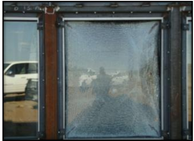
Figure C.24: Specimen 14 External Post-Blast Condition
