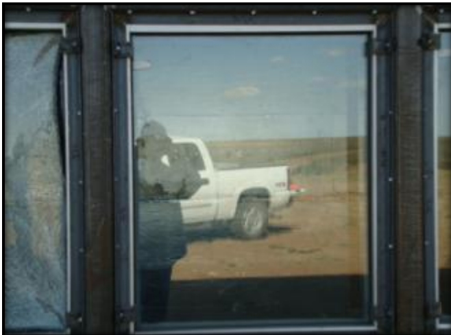
Figure C.25: Specimen 15 External Post-Blast Condition
