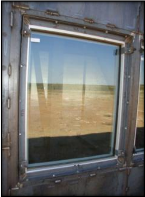
Figure C.1: Specimen 9 Pre-Blast Condition
