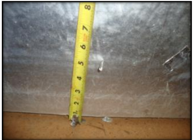
Figure C.8: Glazing Fragment Chamber 3
