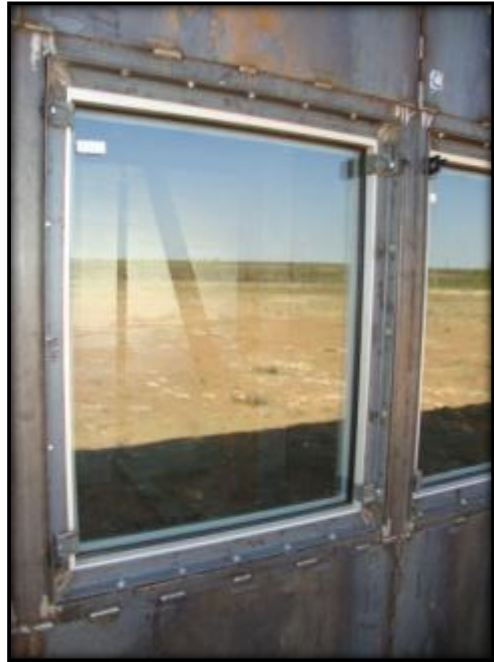
Figure C.2: Specimen 10 Pre-Blast Condition
