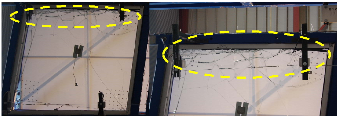
Figure 4.9 Stress concentrations along the top edge of the glass (5'x5' panel with 2-ply 8mil film and wet glazing attachment system subjected to Monotonic load protocol)
