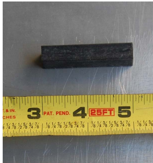
Figure 2.16 Rubber blocks in window units: (a) schematic of general locations and (b) photograph of rubber stop.
