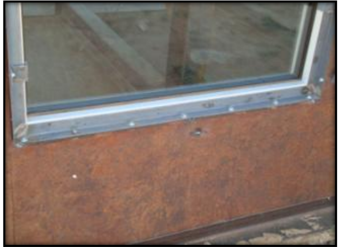
Figure C.2: L1 Bolt Connection Pre-Blast Condition
