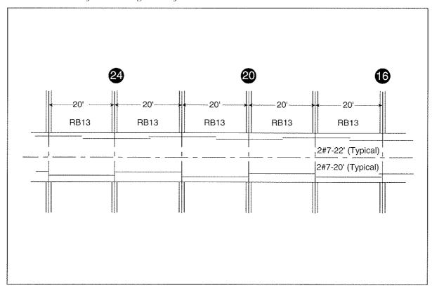
Figure 3-26 Schematic of distorted section showing reinforcing bar arrangement for roof girder at Column Line G.
