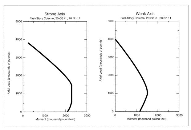
Figure 3-29 Axial load and bending moment capacity for Column G20.
