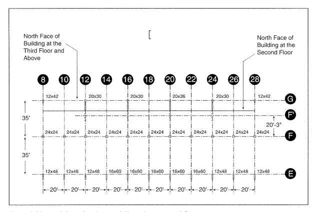
Figure 3-22 Column locations and dimensions – second floor.
