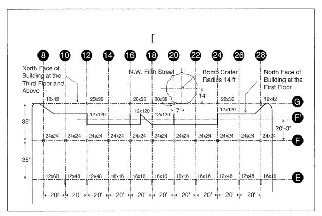
Figure 3-21 Column locations and dimensions – first floor.
