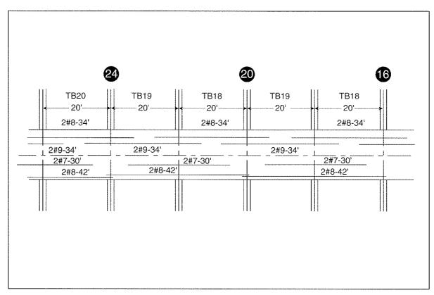
Figure 3-25 Schematic of distorted section showing reinforcing bar arrangement for spandrel girders on fourth through ninth floors at Column Line G.
