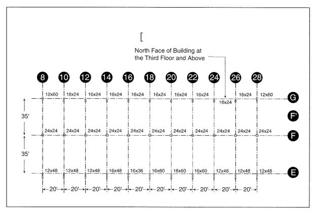
Figure 3-23 Column locations and dimensions – third floor through roof.
