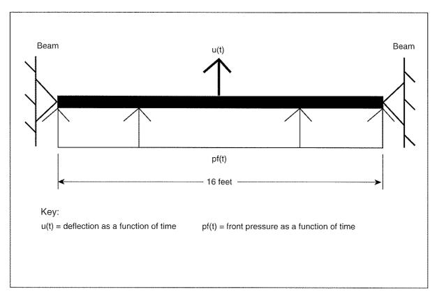
Figure 3-15 Model of slab (single degree of freedom).
