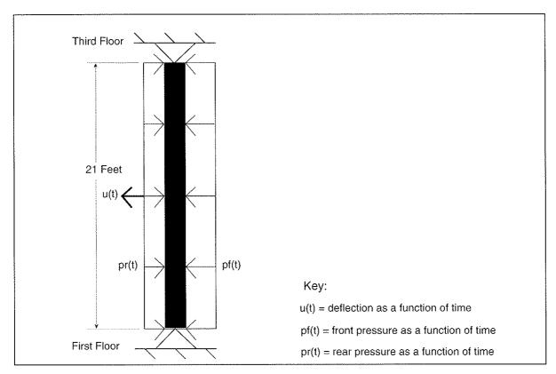
Figure 3-8 Model of Column G24 (singe degree of freedom).
