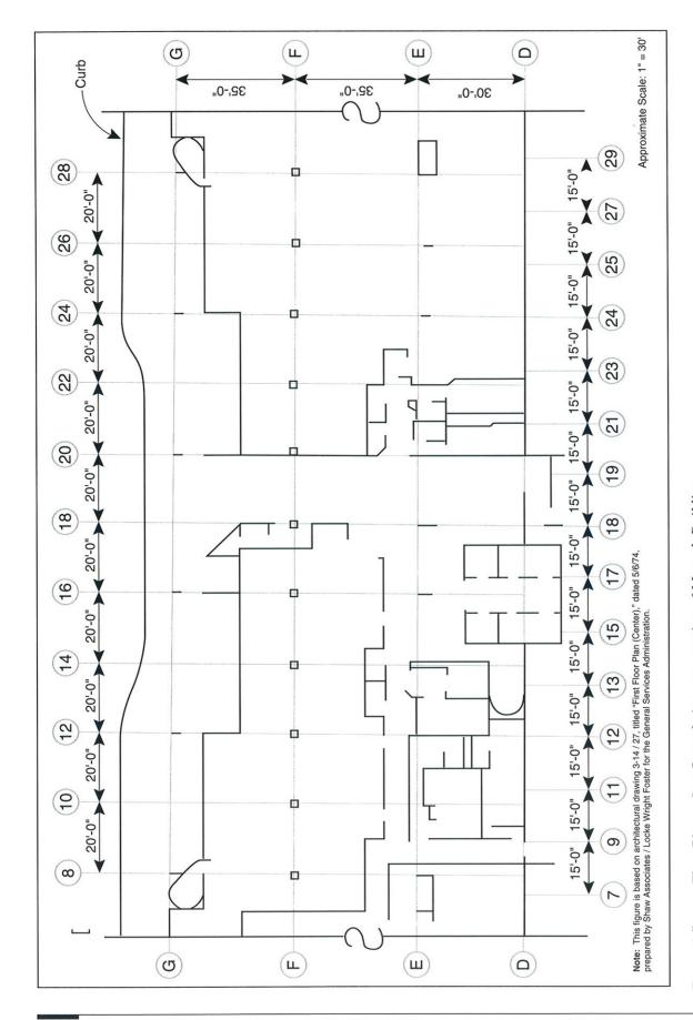
Figure 1-5 Floor Plan – first floor of nine-story portion of Murrah Building.
