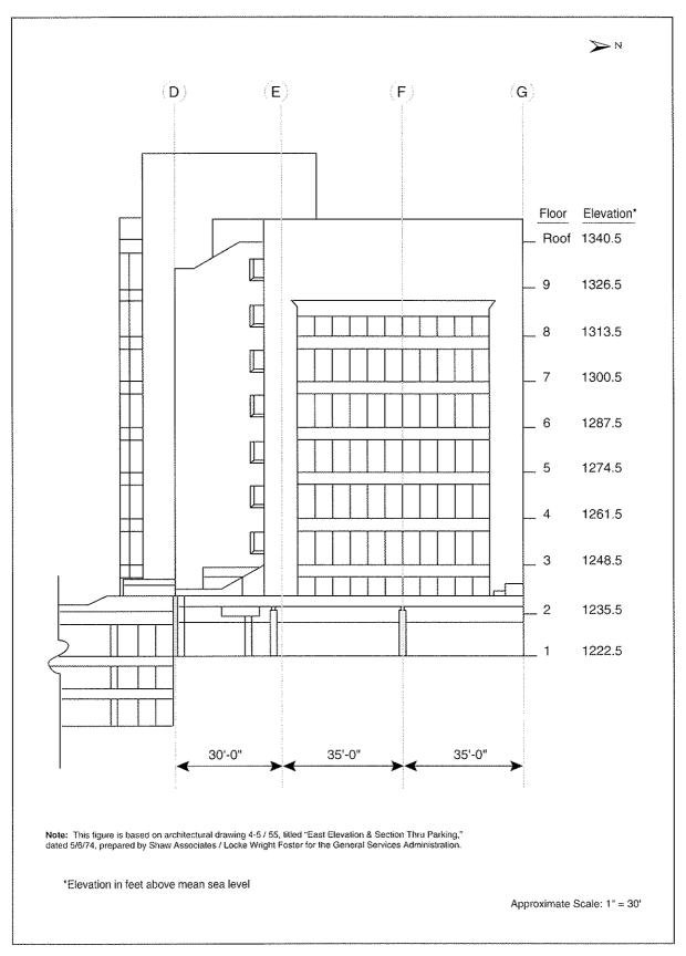
Figure 1-11 East elevation – nine-story portion of Murrah Building.
