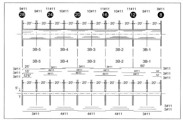
Figure 3-24 Schematic of reinforcement for transfer girder on third floor at Column Line G.
