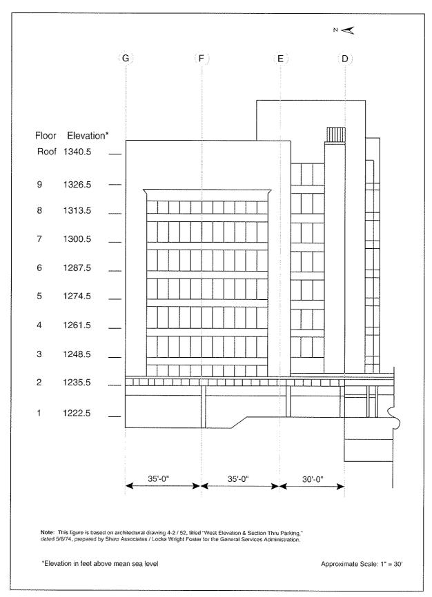
Figure 1-12 West elevation – nine-story portion of Murrah Building.
