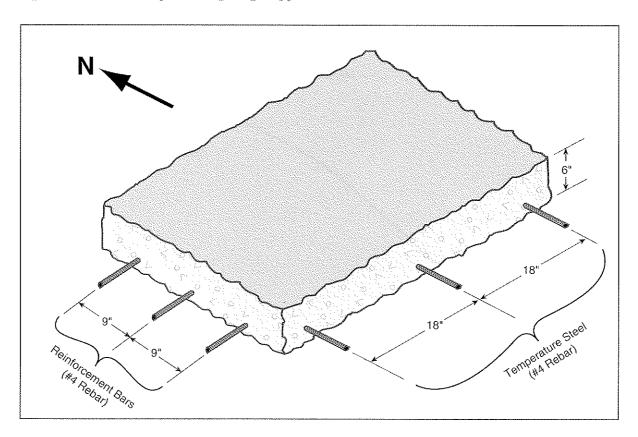
Figure 3-16 Typical section of floor slab at centerline of span.
