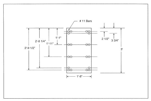
Figure 3-28 Cross section of Column G20 at first floor.
