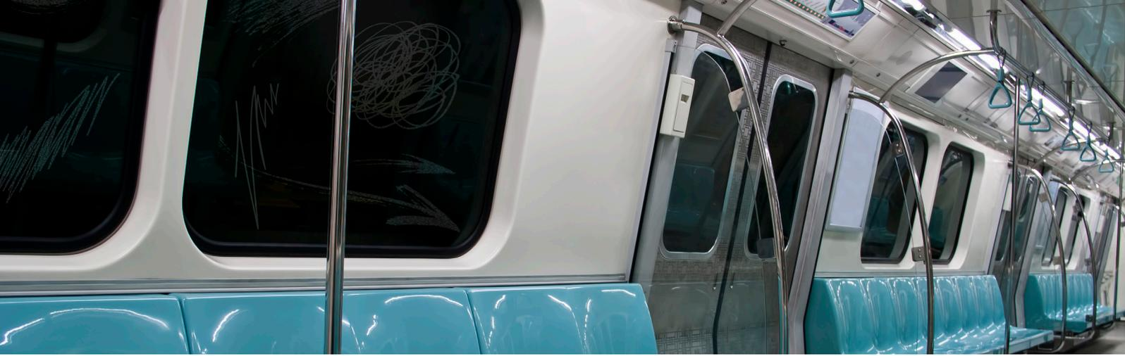
Glass surfaces are common targets for taggers using various tools to scratch or etch their 'art' leaving sometimes irreparable damage. Replacement or repair options can be time consuming and very costly.
