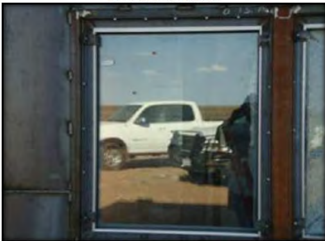
Figure C.21: Specimen 13 External Post-Blast Condition
