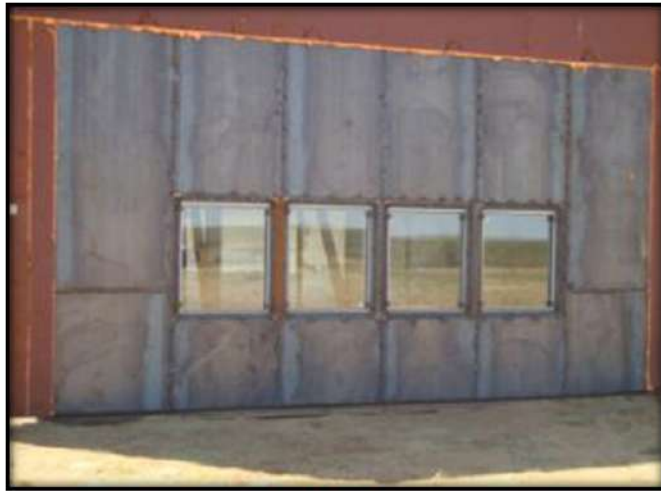
Figure B.5: Pre-Blast Specimen Setup Chamber 4
