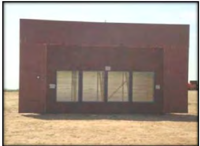
Figure B.4: Pre-Blast Specimen Setup Chamber 1
