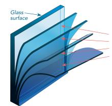
Stack of 4 clear polyester films 100 µm each with opticaly clear removable adhesive and special anti-graffiti hardcoat
