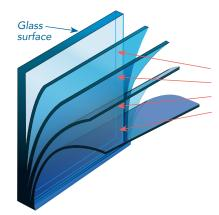
Stack of 4 clear polyester films 100 µm each with opticaly clear removable adhesive and special anti-graffiti hardcoat
